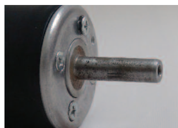
6. Putting screws back in place. Note diagonal tightening of screws.
