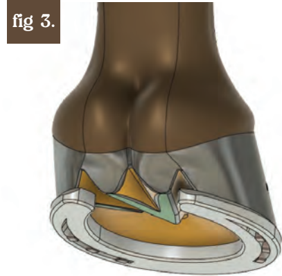
fig 3. A foot shod with a conventional shoe is an extension of the hoof wall. There is an increased load on the hoof wall, and heels are loaded more, the frog and bars are elevated and loaded less.
