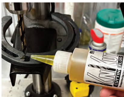
Cutting Fluid applied before drilling
