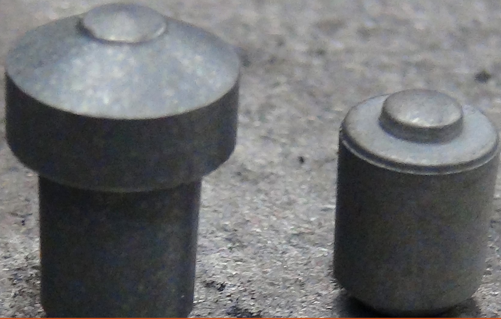
FOOTPRO C11 and C13 SOLID CARBIDE STUDS C11 (left) C13 (right). Both require a 17-64" drill bit.
