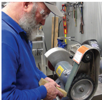
To clean belt, place rubber cleaning stick on belt at a 45° angle.
