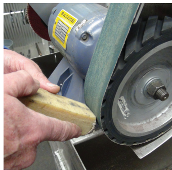
To clean belt, place rubber cleaning stick on belt at a 45° angle.
