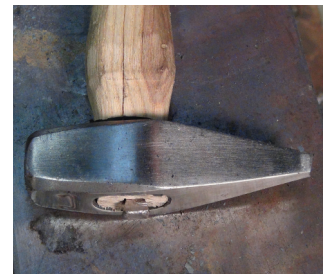
Damaged Wood Handled Forepunch. No heat signature at tip, E-head "wedge" split handle.
