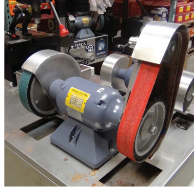
1/2 HP Baldor from FPD with 2x36 FootPro Attachment arm (shown with 36 grit belt) and 10" Expander Wheel.
