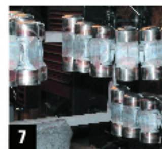
Photo 1: Forging area. Photos 2-6: Forging punches on power hammer. Photo 7: Hammers following heat treat. Photo 8: Grinding tong reins.
