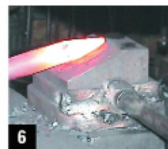
Photo 1: Forging area. Photos 2-6: Forging punches on power hammer. Photo 7: Hammers following heat treat. Photo 8: Grinding tong reins.
