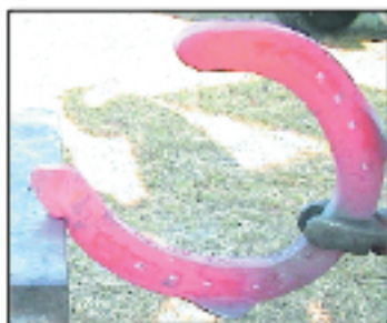
LEFT: About 1" over anvil to set angle; RIGHT: Modify second heel.
