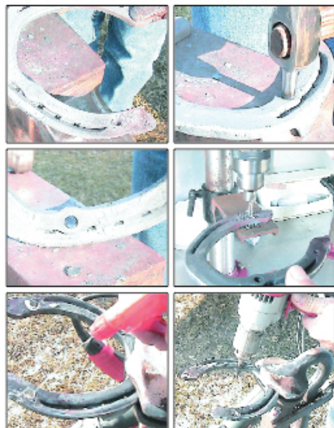
TOP LEFT: From ground surface; TOP RIGHT: Punch through at black heat; ROW 2, LEFT: Punched hole ready to tap; ROW 2, RIGHT: Drilling heels; ROW 3, LEFT: Tapping solution; ROW 3, RIGHT: Tap shoe, use vise to hold secure; BOTTOM: Finished shoe, ready for studs.
