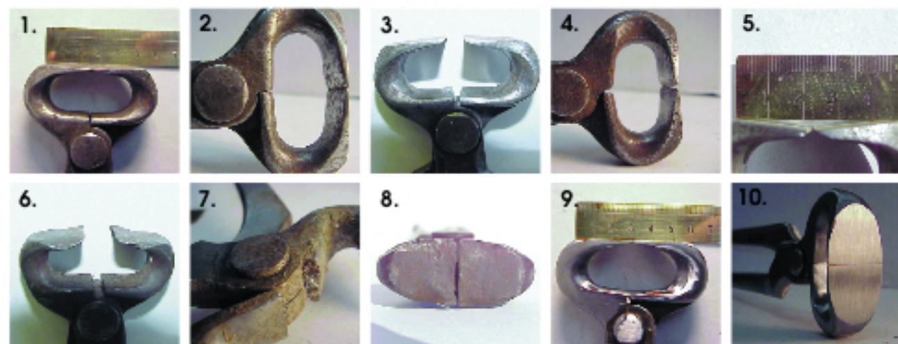
1,2 & 3. Moderate wear, good time to rebuild. 4. The blades make contact but stop doesn't, notice uneven cut. 5 & 6. Severe wear, may not be salvaged. 7. Stop
