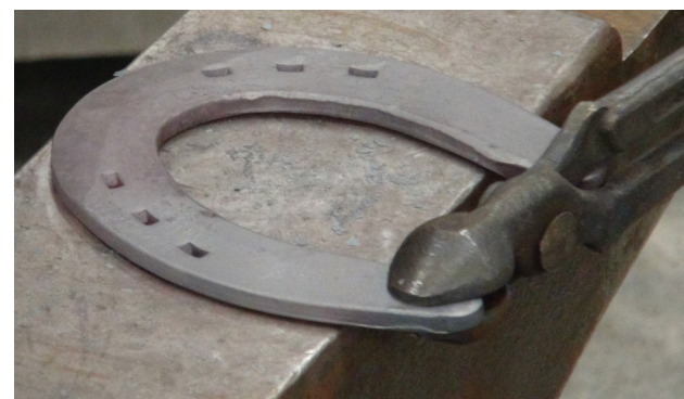
Pride 1" Rolled Toe Modification
