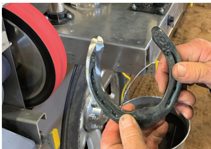
Medial heel ground to allow for sinking in the surface.
