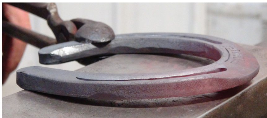
Resulting bevel side view.
