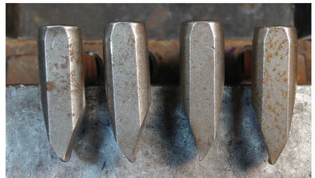
FOUR TOOLS ALL USED IN CROSSOVER STYLE. TWO TOOLS USED BY RIGHT HANDER, TWO BY LEFT HANDER. IF YOU LOOK CAREFULLY YOU CAN SEE ALL WERE STRUCK OFF CENTER.
