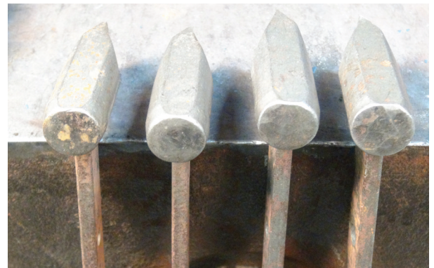
LEFT HANDER USED THIS IN CROSSOVER STYLE. NOTE DAMAGE TO FULLER END.
