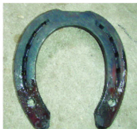
ABOVE: FRONT SHOE, SHAPED, DRILLED AND TAPPED.
