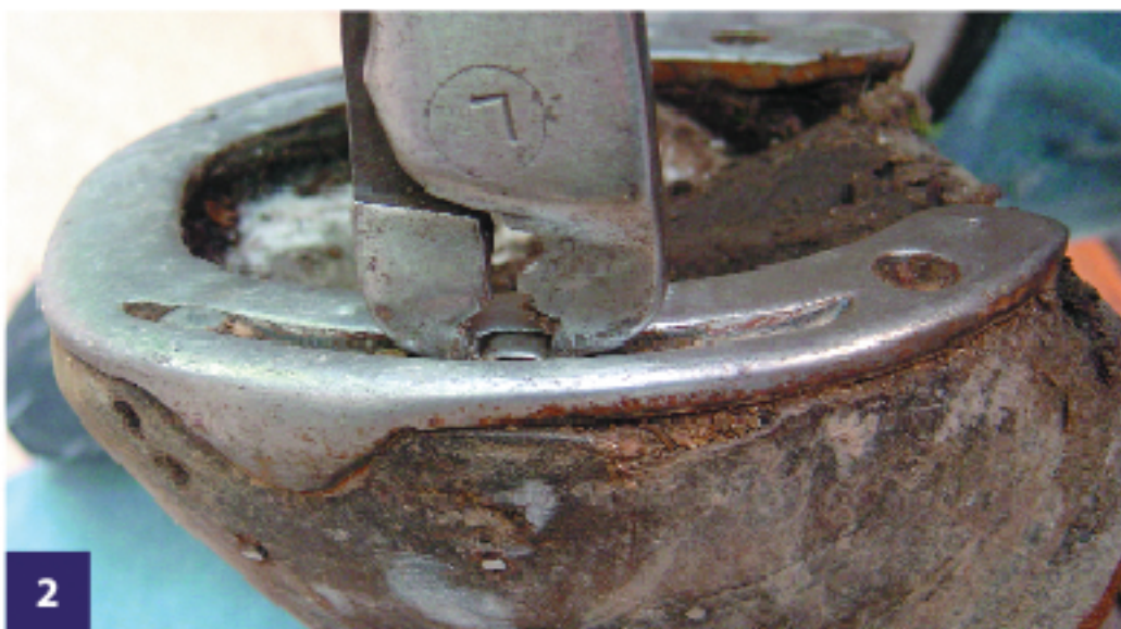
Puller tips are not under nail head; this method causes damage to tool.
