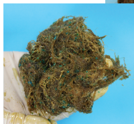
Fig. 4 & 5 - The preferred packing of the EPS at VMCVM is a mixture of oakum, venice turpentinea and copper sulfate.
