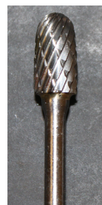
Fig. 7 - Carbide cross cut burrs c .
