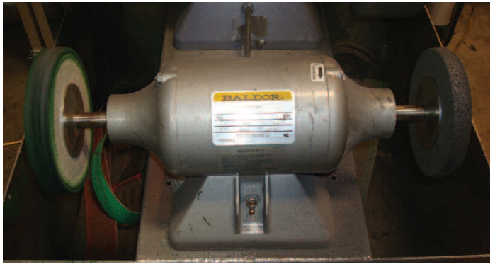
ABOVE: 1/4HP BUFFER WITH SHARPENING WHEEL ON RIGHT AND FELT WHEEL ON LEFT.
