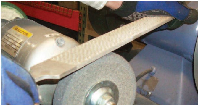
ABOVE: CONTINUE WITH PROCESS UNTIL WHEEL IS EVEN AND DAMAGED AREA IS TAKEN OUT.
