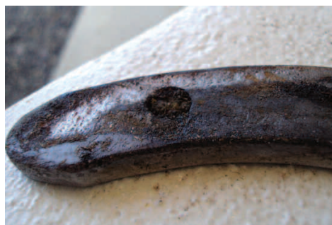
Heel cupping on hoof surface of shoe.
