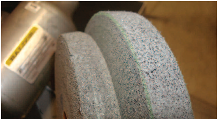
ABOVE: COMPARE DAMAGE AND WEAR TO NEWER WHEEL.
