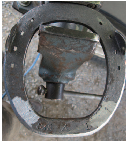
Figure 4. Welds smoothed with a grinder and the heel base is boxed.
