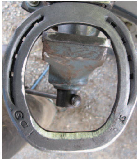
Figure 5. Leading edge of the bar is beveled with a grinder to remove "drag" and allow the foot to slide on impact.
