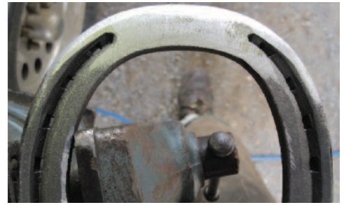
Figure 6. Breakover is created in the shoe with a grinder beginning at the inner margin of the shoe at the toe.
