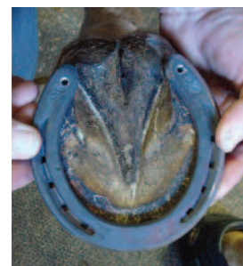
Shoe fit, drilled for pad rivets
