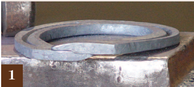
Above: Chain link scarf Below: Step scarf
