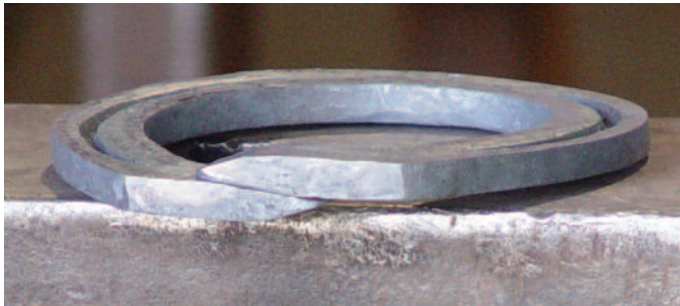
Above: Chain link scarf Below: Step scarf
