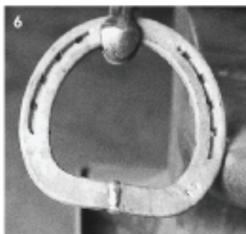
Photos 1-6: When preparing shoes for mig, arc or torch welding, bringing the two ends together is the goal. Don't be concerned with the shape of the shoe at this point.
