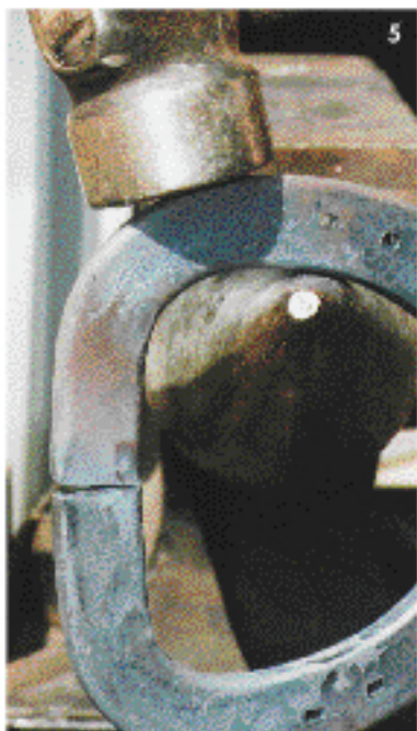
Photos 1-6: When preparing shoes for mig, arc or torch welding, bringing the two ends together is the goal. Don't be concerned with the shape of the shoe at this point.
