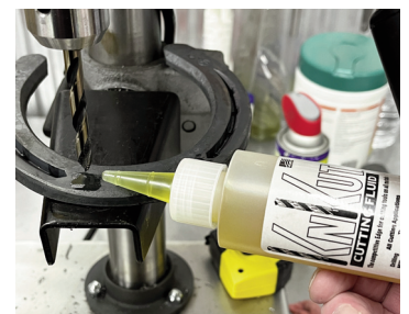
Cutting Fluid applied before drilling
