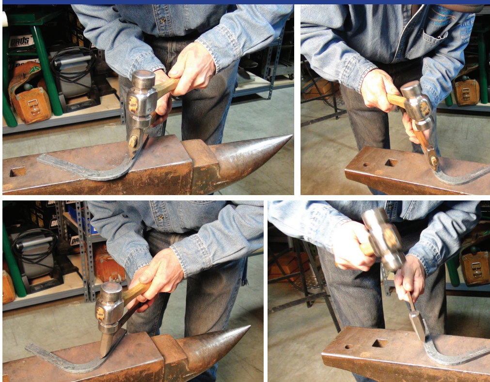
LEFT AND RIGHT HAND INLINE STYLE. LOOK CLOSELY AT THE POSITION OF THE ELBOWS IN RELATION TO THE BODY.
