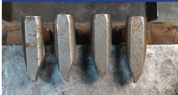
FOUR TOOLS ALL USED IN CROSSOVER STYLE. TWO TOOLS USED BY RIGHT HANDER, TWO BY LEFT HANDER. IF YOU LOOK CAREFULLY YOU CAN SEE ALL WERE STRUCK OFF CENTER.
