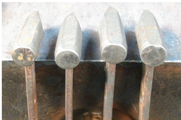
FOUR TOOLS ALL USED IN CROSSOVER STYLE. TWO TOOLS USED BY RIGHT HANDER, TWO BY LEFT HANDER. IF YOU LOOK CAREFULLY YOU CAN SEE ALL WERE STRUCK OFF CENTER.
