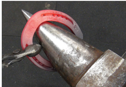
Kerckhaert's hind patterns generally need very little shaping to get ready for nailing. Note the built-in full toe width on all the SX-10's (front and hind).
