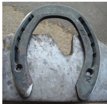
The shoe ground, drilled and tapped.
