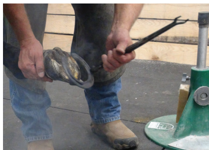
Hot fitting off the stand but notice the aluminum plate modification on the Hoofjack base used to set the hot shoe on while final paring the sole.
